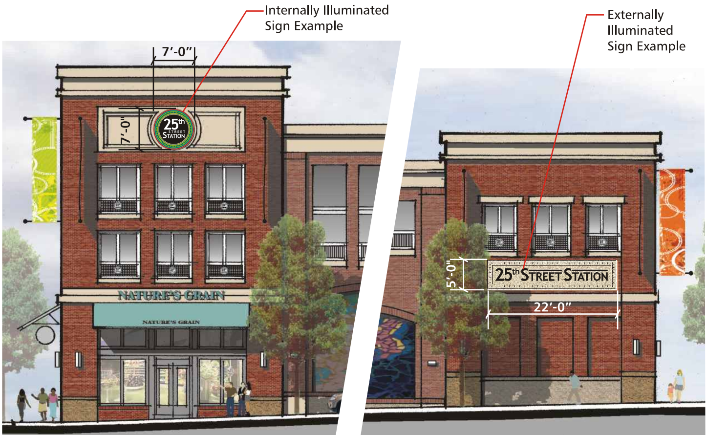
Examples: North Elevations @ Building B2 (W 24th Street)
