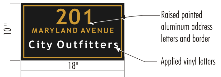
CONDITION #1: SERVICE ENTRY SIGN DETAIL Not To Scale (Message shown as example only)
